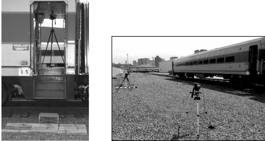
Figure 15. Car #237: Side-Door Stairway – Interior and Exterior Video Cameras
