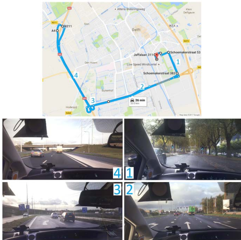
Fig. 1. The driving route in the experiment covering mixed urban and highway roads. Representative screen shots are provided for various route segments at labeled points on the map.
