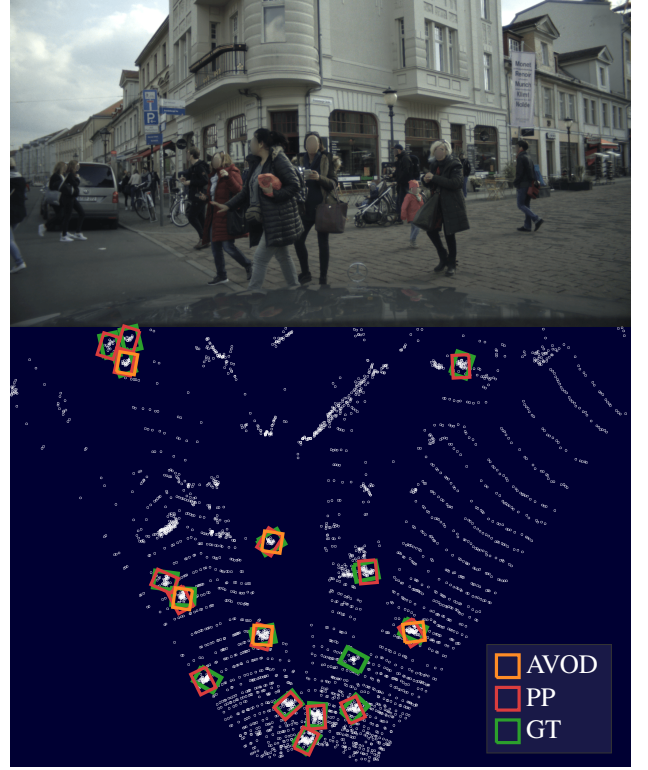
Fig. 1. An example of the predicted bounding boxes of PointPillars [6] (PP) and AVOD [7] on a scene from the EuroCity Persons 2.5D [8], along with the annotated ground truth (GT).
