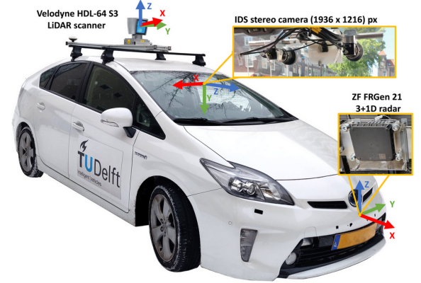
Fig. 2: Recording platform. Our Toyota Prius 2013 platform is equipped with a stereo camera setup, a rotating 3D LiDAR sensor, a ZF FRGen 21 3+1D radar, and a combined GPS/IMU inertial navigation system.
