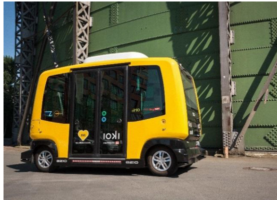
Fig. 2. Automated shuttle 'Emily', EZ10, by Easymile on the EUREF campus in Berlin, Germany.
