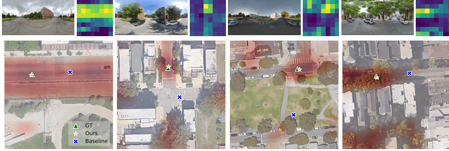
Fig. 11. Qualitative results on VIGOR dataset cross-area split. Top: input ground images and matching score maps at the model bottleneck, bottom: input satellite image overlaid with outputs from CVR and our method.
